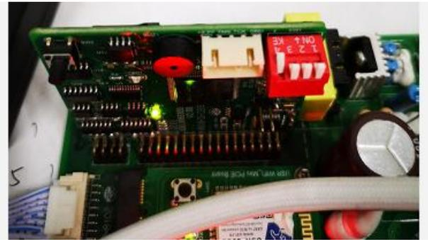
2. Connect the charger to your laptop via network cable(RJ45 cable). The IP of the laptop should be within the same network segment with the EV charger. The charger's default IP address is 192.168.1.5. So you'll need to set the IP of your laptop to 192.168.1.x, (x can be any value between 1 and 255 except 5).
