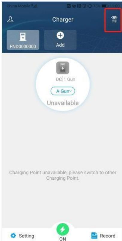
5. Turn on the breaker of the EV charger to power it up, then click “Go to the WLAN page to set up” to connect the mobile phone to the hotspot generated by the charger. The name of the hotspot is the charger’s serial number, the password is 12345678.
